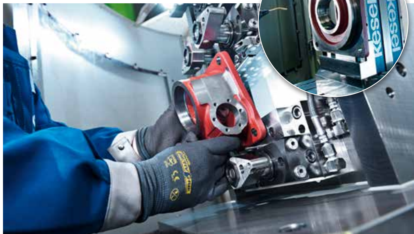
Production Pfaff-silberblau: Worm gear screw jacks housing machining
