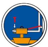
Be sure that the fork sleeves are mechanically fixed (with locking screw and safety chain or rope) to the lifting device.
