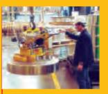
Introduction of the first coil lifters for the transport of split strip rings
