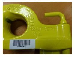
The reverse of the lug has the loading for lifting frame use.
