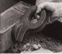
3) Turn lug until spring bolt is fully engaged in slot.
